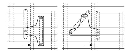
Access is normally achieved by removing a section of floorboard adjacent to the fixing area large enough to allow the insertion and positioning of the bars. All floorboards taking any part of the load should be securely fastened down to the joists with 4" (100mm) countersunk wood screws. The final installation should be tested according to the manufacturers recommendations.
