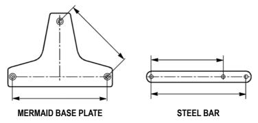
All three holes in the base plate should be used, with one bar spanning either 'A' or 'B' and the other bar bolted through the third hole. Three countersunk steel screws are supplied for this purpose. Ideally each bar should span as many floorboards as possible (usually three). Whether a bar will span either 'A' or 'B' will be decided according to the direction and position of the joists in the area chosen for siting the Bath Lift.
